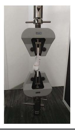
FIGURE 3. Tibia model with implanted plate on Llyod-Ametek EZ-50 Material Testing Machine.
